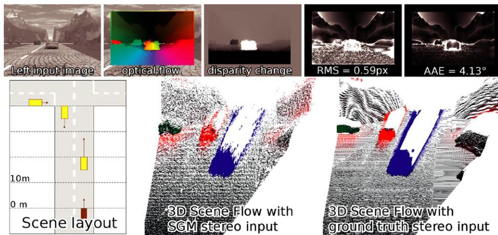
**Fig. 12** (Color online) Povray-rendered traffic scene (Frame 11). *Top*: Colour encodes direction (border = direction key) and intensity the magnitude of the optical flow vectors. *Brighter areas* in the error images denote larger errors. For comparison, running the code from Huguet and Devernay (2007) generates an RMS error of 0.91 px and
