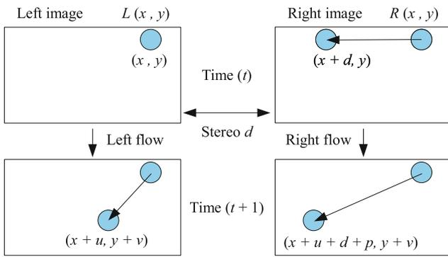
**Fig. 3** Motion and disparity constraints employed in our scene flow algorithm. Intensity consistency of corresponding points in the left and right stereo image and in successive frames is assumed. This assumption is relaxed later in Sect. 2.5
