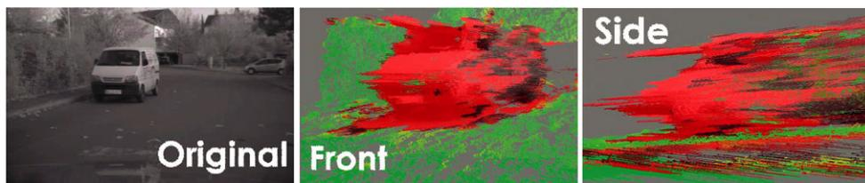
**Fig. 20** (Color online) A real-world example of our scene flow. The left image shows the original, the two other images show the scene flow reconstruction when viewed from the front and side. Colour encoding is green ↔ red is stationary ↔ moving
