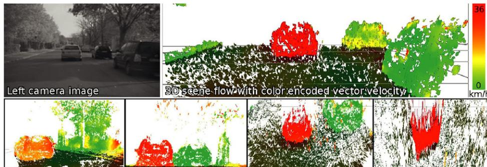
**Fig. 18** (Color online) This figure shows the scene flow results when following another vehicle. *Top row*: shows an original image with the *colour* encoded scene flow. The *bottom row* shows different virtual viewing points on the same 3D scene. *Left to right*: panning to left
