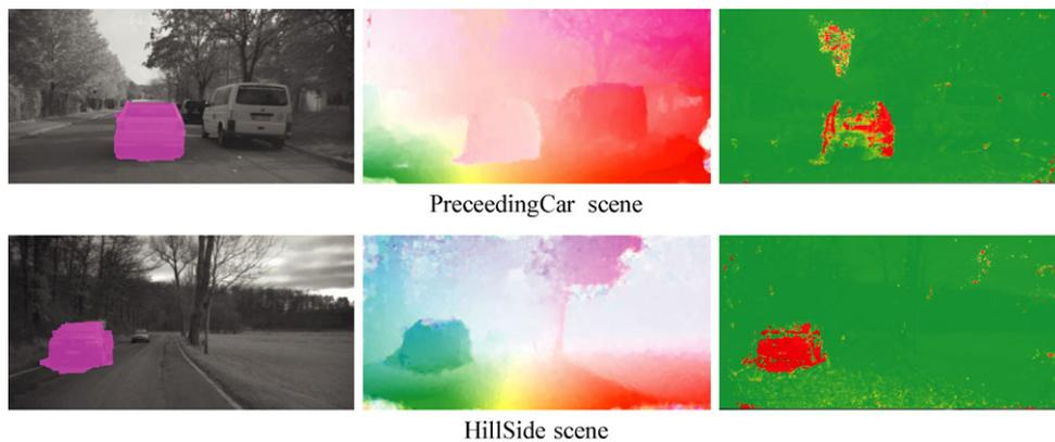
**Fig. 23** (Color online) The figure shows segmentation of independently moving objects moving parallel to the camera movement. This movement cannot be detected monocularly without additional constraints, such as a planar ground assumption. Using our motion likeli-
