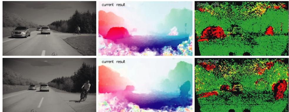
not know of a way to determine whether this correlation is positive or negative. From this model, one can see that the disparity measurement has the highest influence on the covariance (as it is either by itself or quadratically weighted in the equations). Furthermore, the larger the disparity, the more precise the measurement; as  $d \rightarrow \infty$  all  $\sigma_\alpha \rightarrow 0$ .
