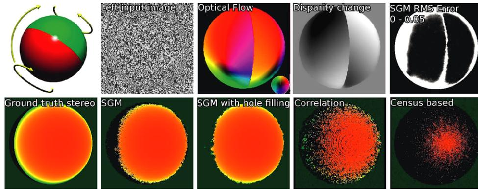
**Fig. 11** (Color online) Ground truth test: *rotating sphere*. Quantitative results are shown in Table 2. *Top*: The *left image* shows the movement of the sphere. Optical flow and disparity change are computed on the basis of SGM stereo (Hirschmüller 2008). *Colour* encodes the direction of the optical flow (key in *bottom right*), intensity its magnitude.
