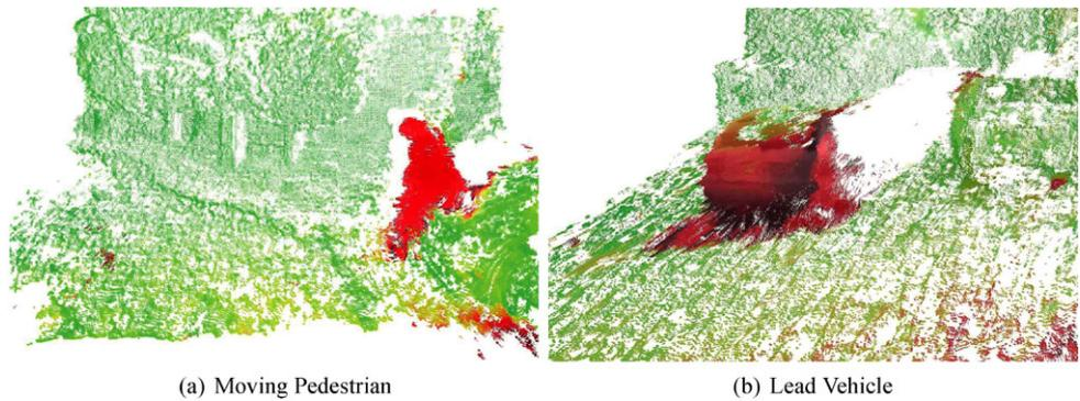
**Fig. 9** (Color online) Two examples, from a single sequence, of the residual motion likelihood defined in Sect. 4.1. Left to right: original image, optical flow result, the residual motion metric results ( $green \leftrightarrow red$  represents low  $\leftrightarrow$  high likelihood that point is moving)
