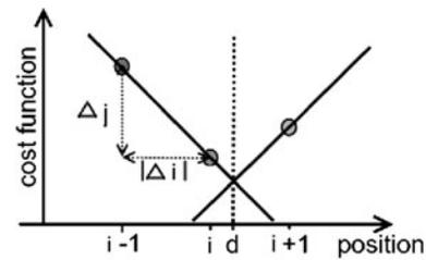
**Fig. 6** Quality measure for the disparity estimate. The slope of the disparity cost function serves as a quality measure for the disparity estimate
