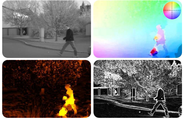
Figure 2. Optical flow estimation for a scene with a running person. Even the large displacement of the right foot is correctly matched. The lower images show the \rho_{\mathbf{F}} constraint deviations which clearly identify the person and the edge image |\nabla I| .
