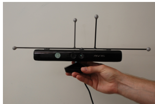
(c) Microsoft Kinect sensor with reflective markers
