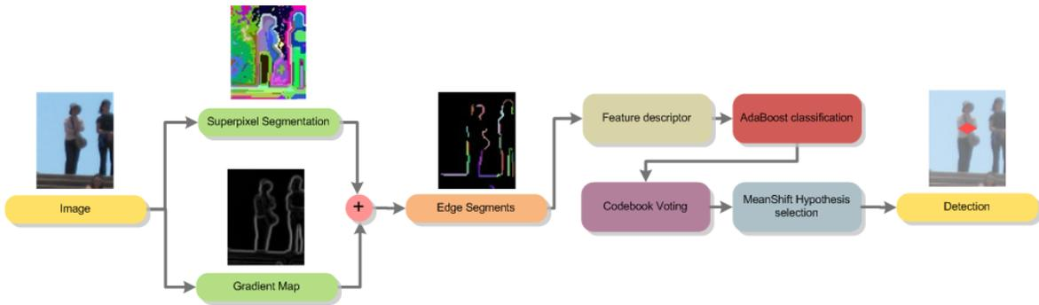
Fig. 2. Flowchart of our detection algorithm.
