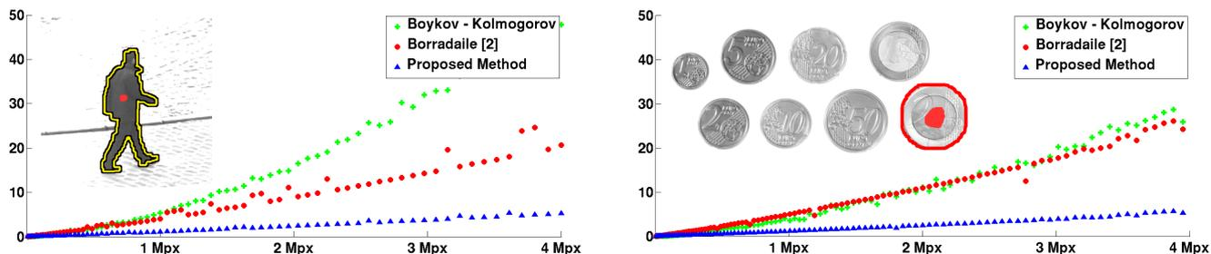
**Figure 4. Runtimes of image segmentation.** The runtime on the  $y$ -axis is measured in seconds and depends on the resolution of the images. The proposed approach is faster than the method of Boykov and Kolmogorov. Also, it has a much smaller runtime spread for different images and the observed speed-up increases at higher image resolutions.
