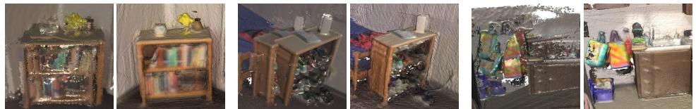
Figure 9: Qualitative comparison of ElasticFusion [21] (left) with our method (right) on *BundleFusion/apt0*. The point cloud reconstructed with ElasticFusion exhibits artifacts due to potentially undetected loop closures and surface warping artifacts, whereas our method successfully corrects the model.
