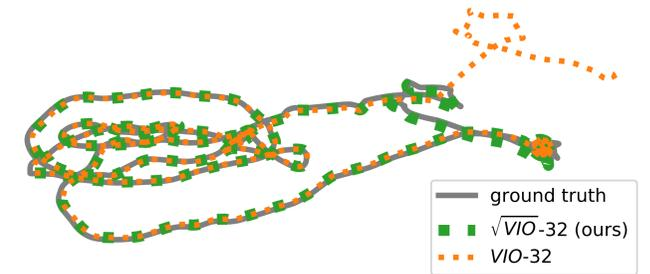
The conventional baseline VIO-64 works well with double-precision floats, but fails in single precision (VIO-32). In contrast, the proposed square root estimator  $\sqrt{VIO-32}$  even in single precision retains the same accuracy.
