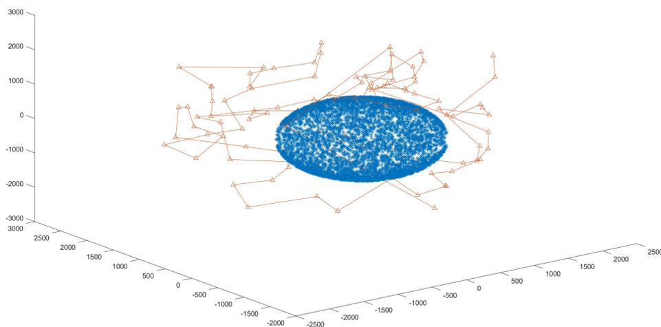
Figure 5.2: Synthetic dataset with 100 image frames and 5000 feature points in system  $O$ . The feature points are presented by blue ”\*”; and the camera locations are presented as red ” $\Delta$ ”. All camera locations are connected together with red line according to its arranged order.
