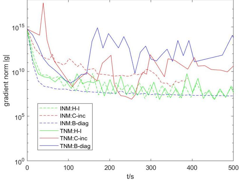
Figure 3.13: Comparison of the gradient norm curves between INM implementations and TNM implementations. In general, INM implementations have a deeper and more stable reduction of the gradient norm related to TNMs.
