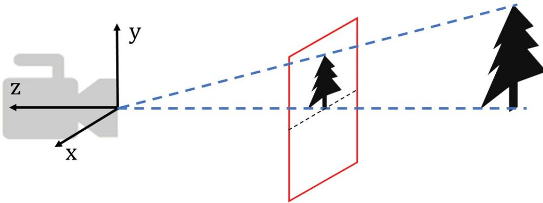
Figure 2.2: Perspective projection in a camera system. The red plane presents the projection plane located at  $(0, 0, -f)$ . The real 3D object (tree) is proportionally projected onto this plane.
