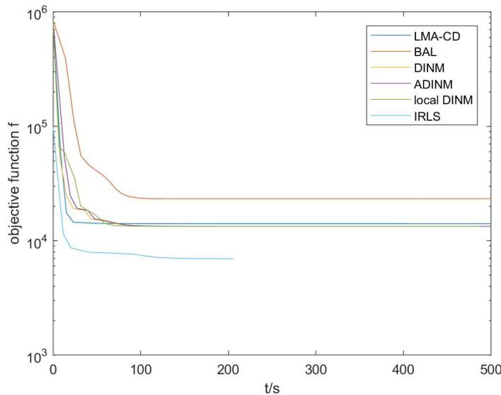
Figure 5.6: Comparison of the objective function curves between our implementations and baseline implementations running on the Ladybug dataset provided by [ASSS] with 49 image frames, 7776 feature points, and 31843 observations. "DINM", "ADINM", and "local DINM" obtain the smallest value of the objective function.
