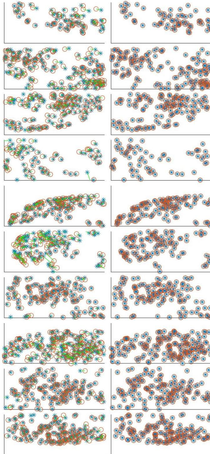
Figure 5.5: The reprojection errors on the small-scale synthetic dataset. The results are plotted in all 10 image frames. The first column presents the reprojection at the initialization; the second column presents the reprojection after 100 iteration steps of "DINM:inc-I".
