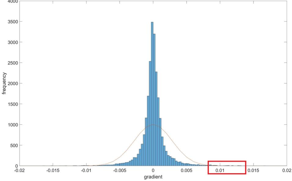
Figure 4.6: The frequency histogram of gradients after 50 iteration steps of ADINM. The orange curve presents the Gaussian probability distribution function with the same mean and variance. The example red rectangle locates the outliers, where the frequency of reprojection errors is higher than corresponding Gaussian distribution.
