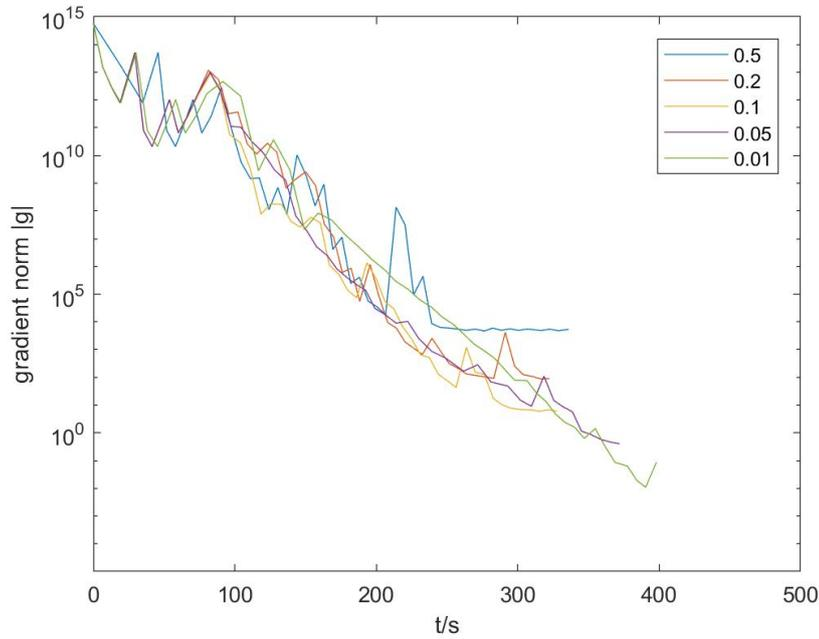
Figure 3.23: Comparison of the gradient norm curves between different termination factors in PCG loop in DINM implementations. The gradient norm has a more stable reduction with a smaller number of the termination factor, but a too small number also causes a long computation time. A proper termination factor can be set to a value around  $0.05 \sim 0.1$ .
