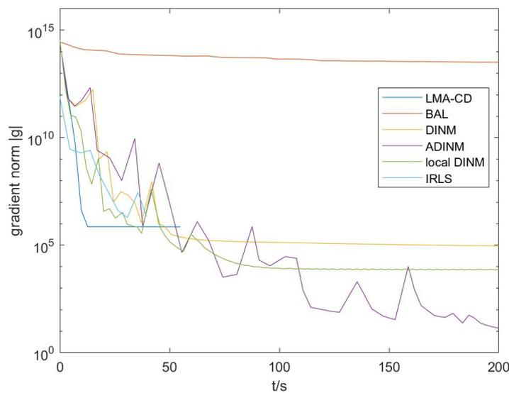
Figure 5.13: Comparison of the gradient norm curves between our implementations and baseline implementations running on the medium-scale synthetic dataset with 50 image frames, 1000 feature points, and 28991 observations. "ADINM" has the fastest and the deepest decline of the gradient norm.
