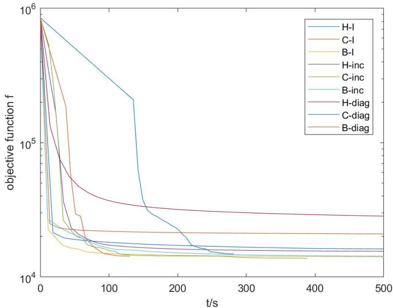
Figure 3.8: Comparison of the objective function curves between different INM implementations. "H" represents without Schur complement; "C" represents Schur complement of  $\mathbf{C}$ ; "B" represents Schur complement of  $\mathbf{B}$ . "inc" represents scaling matrix formed from (3.38); "diag" represents scaling matrix formed from the diagonal of Hessian matrix; "I" represents without scaling, i.e. scaling matrix is identity matrix. "C-inc" has the smallest value of the objective function.
