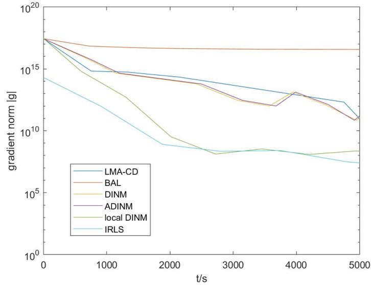
Figure 5.19: Comparison of the gradient norm curves between our implementations and baseline implementations running on the large-scale synthetic dataset with 500 image frames, 5000 feature points, and 1477513 observations. "local DINM" has the fastest and the deepest decline of the gradient norm.
