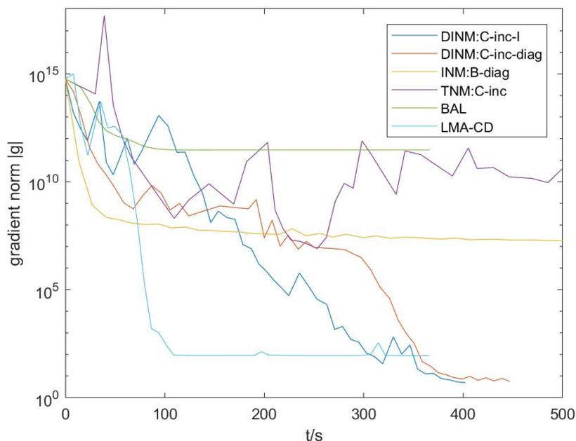
Figure 3.17: Comparison of the gradient norm curves between DINM implementations and INM, TNM and baseline implementations. "inc-I" and "inc-diag" perform better in the gradient decline than others.
