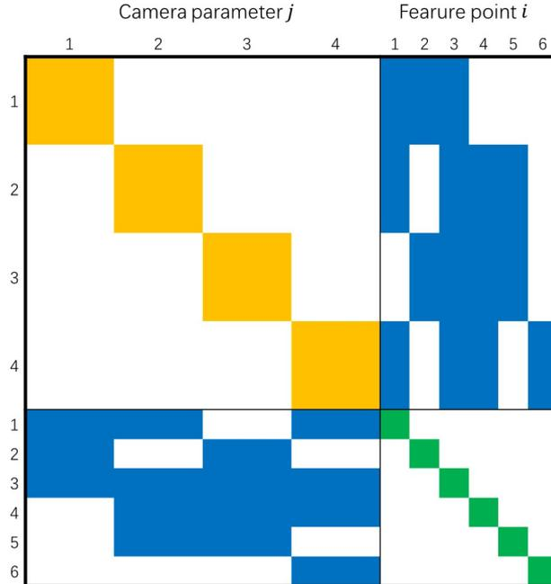
Figure 3.3: Hessian matrix demonstration of a small bundle adjustment problem (same as in Figure 3.2). The yellow block in  $\mathbf{B}$  is of size of  $9 \times 9$ ; the green block in  $\mathbf{C}$  is of size of  $3 \times 3$ ; the blue block in  $\mathbf{E}^T$  is of size of  $3 \times 9$ . If the blue blocks in  $\mathbf{E}^T$  is labeled with index  $(i, j)$ ,  $(i, j)$ -block is a non-zero matrix, if and only if when  $(i, j) \in \mathcal{S}$ .
