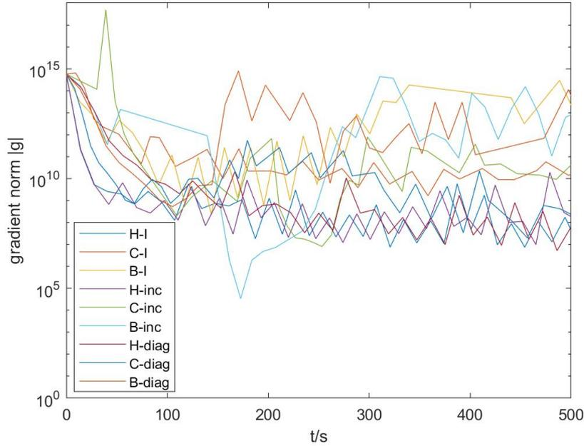
Figure 3.11: Comparison of the gradient norm curves between different TNM implementations. "H-I" has the smallest fluctuation in the gradient reduction.
