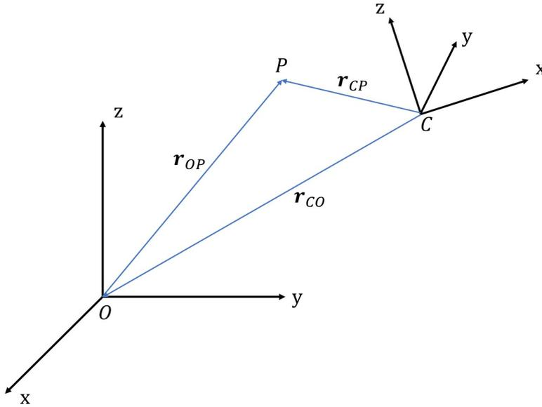
Figure 2.1: 3D coordinates (point  $P$ ) transformation between coordinate system  $O$  and coordinate system  $C$ .
