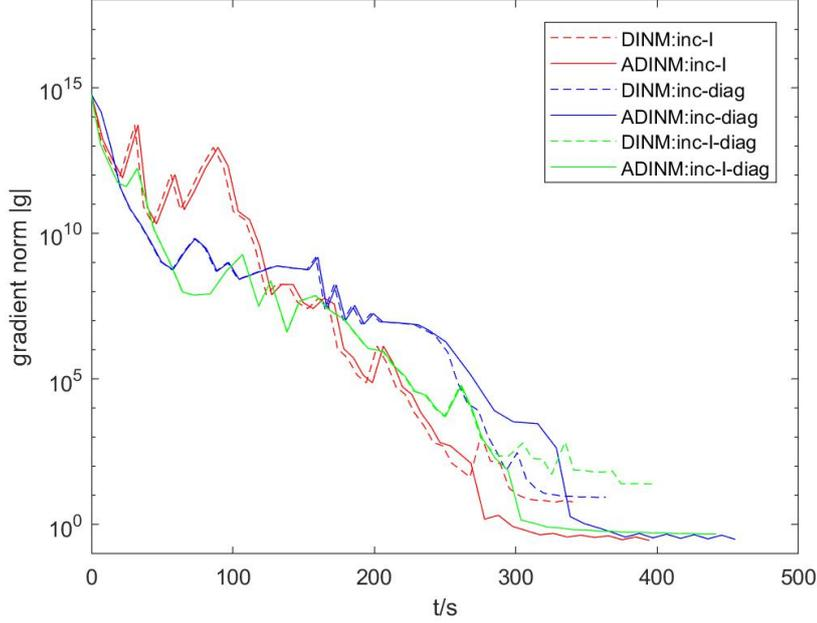
Figure 4.2: Comparison of the gradient norm curve between DINM implementations and corresponding ADINM implementations. ADINM yields a deeper decline curve of the gradient norm than DINM.
