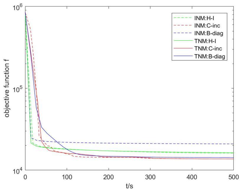
Figure 3.12: Comparison of the objective function curves between INM implementations and TNM implementations. All INM implementations are plotted in dash lines; and their corresponding TNM implementations are plotted in solid lines with the same colors. In general, TNM implementations have a faster and deeper reduction of the objective function related to INMs.
