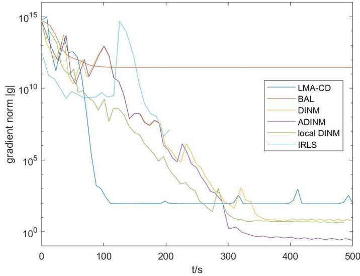
Figure 5.7: Comparison of the gradient norm curves between our implementations and baseline implementations running on the Ladybug dataset provided by [ASSS] with 49 image frames, 7776 feature points, and 31843 observations. "ADINM" yields the deepest reduction curve of the gradient norm.
