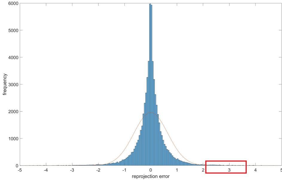
Figure 4.5: The frequency histogram of reprojection errors after 50 iteration steps of ADINM. The orange curve presents the Gaussian probability distribution function with the same mean and variance. The example red rectangle locates the outliers, where the frequency of reprojection errors is higher than corresponding Gaussian distribution.
