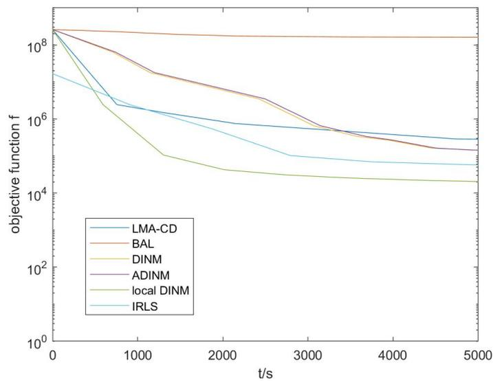
Figure 5.18: Comparison of the objective function curves between our implementations and baseline implementations running on the large-scale synthetic dataset with 500 image frames, 5000 feature points, and 1477513 observations. "local DINM" has the fastest and the deepest decline of the objective function.
