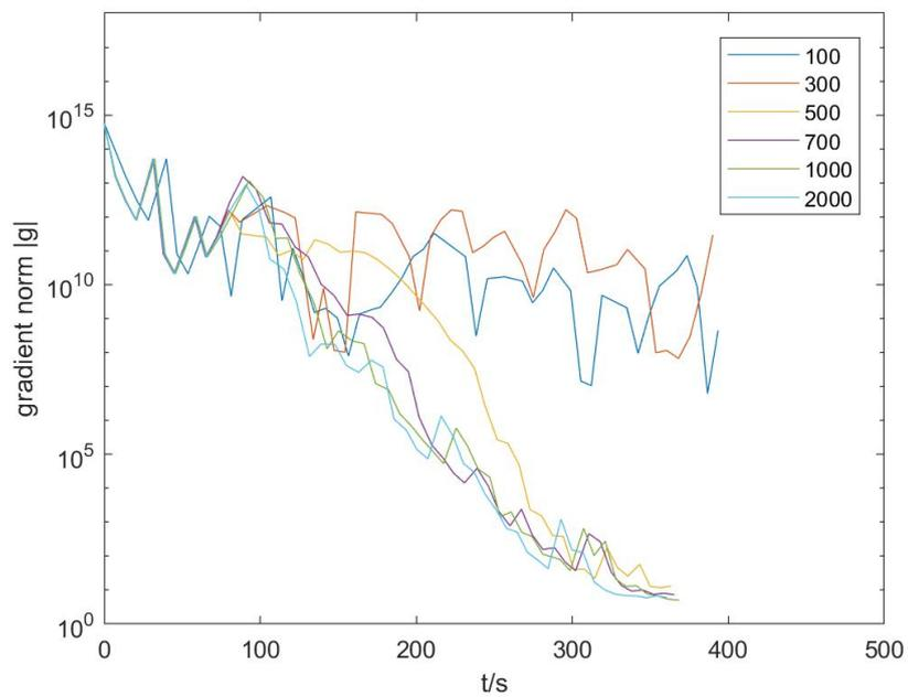
Figure 3.21: Comparison of the gradient norm curves between different iteration steps in PCG loop in DINM implementations. The gradient norm has a faster decreasing with a larger number of maximum iterative steps in PCG loop, and this threshold should be set to a value greater than 700 for this dataset.
