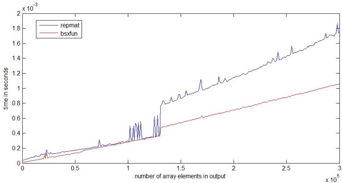
Figure 5.3: Execution time comparing between *repmat* and *bsxfun* in Matlab along the increasing of the scale of the input data. [Jon] *bsxfun* is used in this thesis.
