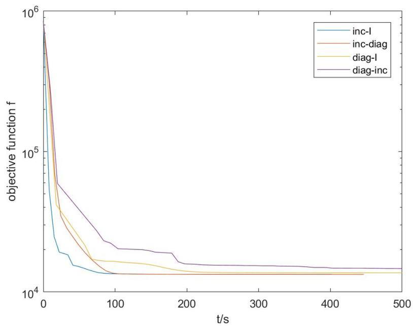
Figure 3.14: Comparison of the objective function curves between different DINM implementations (with different scaling matrix and different damping matrix). For example, "inc-diag" represents, scaling matrix is formed from (3.38), and damping matrix is formed from the diagonal of Hessian matrix. "inc-I" has the fastest and deepest decreasing of the objective function.
