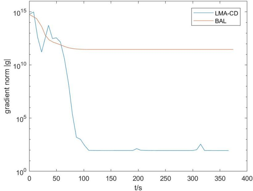
Figure 3.7: Comparison of the gradient norm curves between both baseline implementations. "LMA-CD" performs better in the gradient reduction on the Ladybug dataset.
