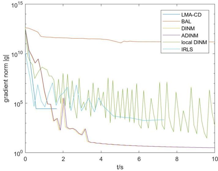
Figure 5.10: Comparison of the gradient norm curves between our implementations and baseline implementations running on the small-scale synthetic dataset with 10 image frames, 289 feature points, and 1834 observations. "DINM" and "ADINM" have the deepest and the most stable decline of the gradient norm.
