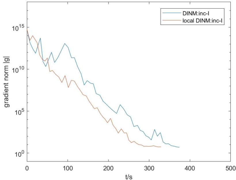
Figure 4.4: Comparison of the gradient norm curve between local and global parameterization. Local parameterization has a little faster reduction curve of the gradient norm.
