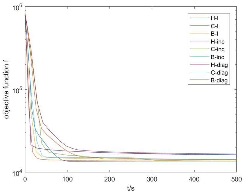
Figure 3.10: Comparison of the objective function curves between different TNM implementations. "H" represents without Schur complement; "C" represents Schur complement of  $\mathbf{C}$ ; "B" represents Schur complement of  $\mathbf{B}$ . "inc" represents damping matrix formed from (3.38); "diag" represents damping matrix formed from the diagonal of Hessian matrix; "I" represents with identity damping matrix. "C-diag" has the smallest value of the objective function.
