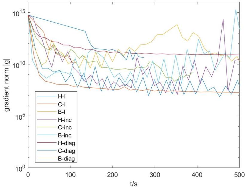
Figure 3.9: Comparison of the gradient norm curve between different INM implementations. "B-diag" performs the best decline curve of the gradient norm.
