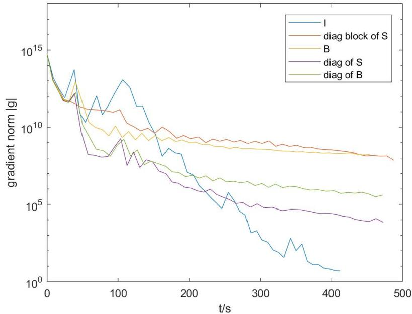
Figure 3.19: Comparison of the gradient norm curves between different preconditioners in DINM implementations. Implementation without preconditioner ("I") yields a faster and deeper decline curve of the gradient norm than others.
