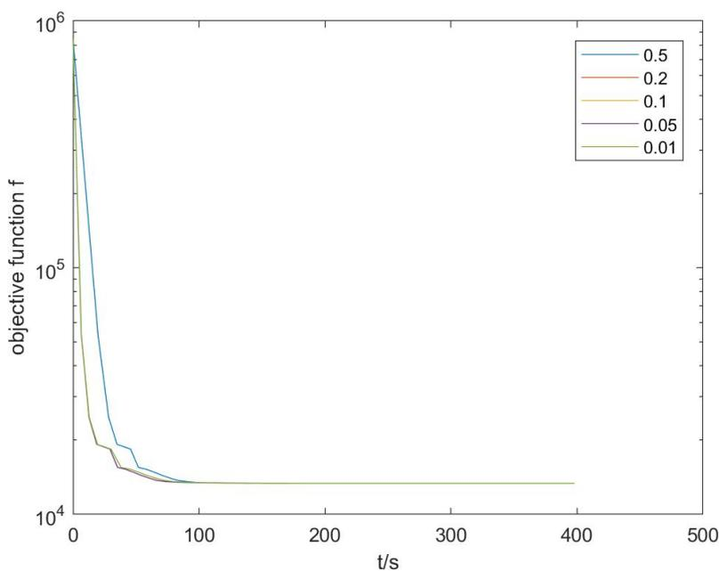
Figure 3.22: Comparison of the objective function curves between different termination factors in PCG loop in DINM implementations. All implementations are based on the algorithm "DINM:inc-I" (seeing the previous section). The number presents the termination factor in PCG loop. All implementations have a similar objective curve.
