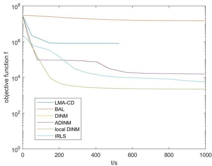
Figure 5.15: Comparison of the objective function curves between our implementations and baseline implementations running on the larger medium-scale synthetic dataset with 100 image frames, 4000 feature points, and 228658 observations. "local DINM" has the fastest and the deepest decline of the objective function.
