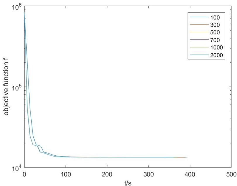
Figure 3.20: Comparison of the objective function curves between different iteration steps in PCG loop in DINM implementations. All implementations are based on the algorithm "DINM:inc-I" (seeing the previous section). The number presents the maximum iteration steps in PCG loop. All implementations have a similar objective curve.
