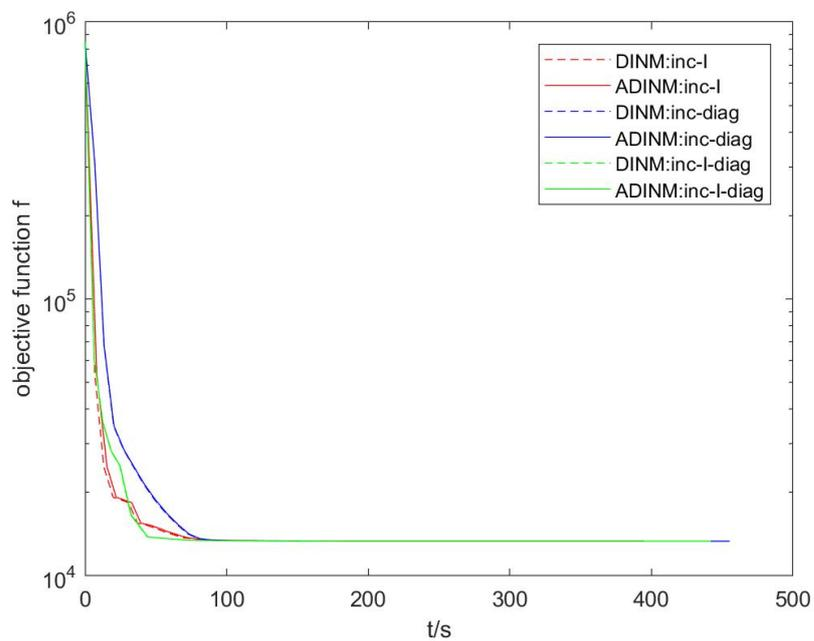
Figure 4.1: Comparison of the objective function curve between DINM implementations and corresponding ADINM implementations. Every DINM implementation and its corresponding ADINM implementation are grouped together with the same color of curves. DINMs are plotted in dash lines; ADINMs are plotted in solid lines. Both ADINM and DINM have a similar reduction curve of the objective function.
