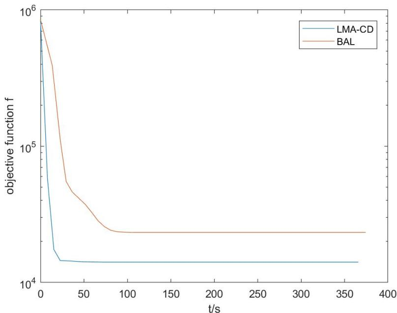
Figure 3.6: Comparison of the objective function curves between both baseline implementations. "LMA-CD" performs better in the objective function reduction on the Ladybug dataset.
