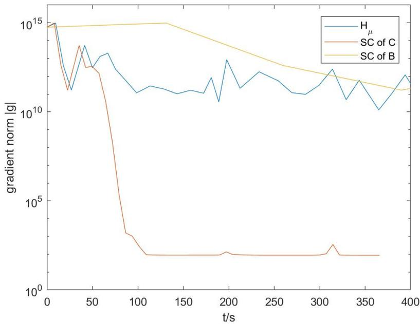
Figure 3.5: Comparison of the gradient norm curve between different Schur complement in LMA solved by Cholesky decomposition. The implementation with SC of  $C$  has the best performance, and stands for "LMA-CD" in the following.
