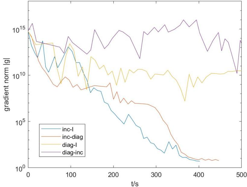
Figure 3.15: Comparison of the gradient norm curves between different DINM implementations. "inc-I" and "inc-diag" perform better in the gradient decline than others.
