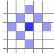
Figure 4: Neighborhood pattern used to compute the objective cost in PBA ([1]).
