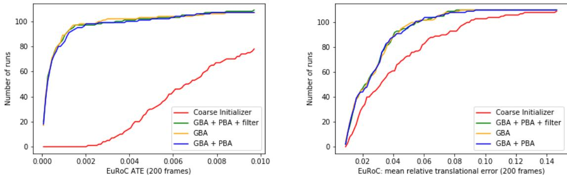
Figure 18: EuRoC: cumulative plot for trajectory errors, ORB Initializer versions comparison (only keyframes) [ $m^{-1}$ ].
