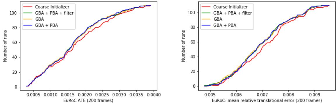
Figure 20: EuRoC: cumulative plot for trajectory errors, ORB Initializer versions comparison (over 200 frames) [ $m^{-1}$ ].
