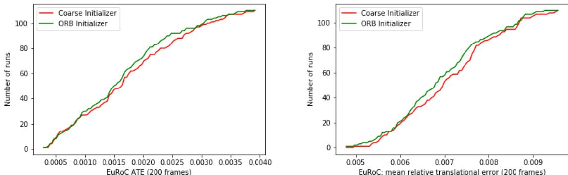
Figure 19: EuRoC: cumulative plot for trajectory errors (over 200 frames) [ $m^{-1}$ ].
