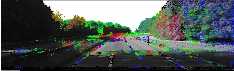
Figure 1: Example of inverse depth map initialization with KITTI sequence 01 (red patches indicate close to camera points, blue - far away ones).
