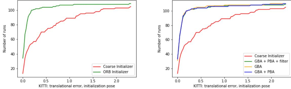
Figure 11: KITTI: cumulative plot for initial keyframe pose [ $m^{-1}$ ].
