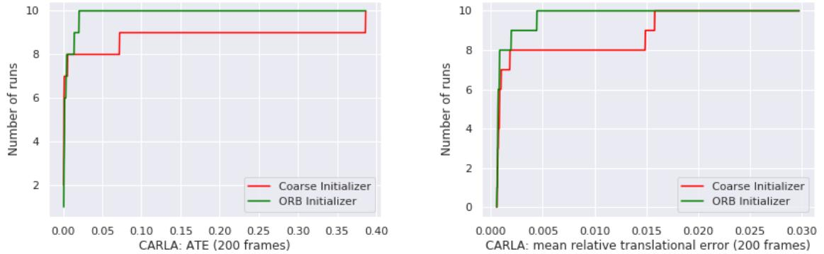
Figure 9: CARLA: cumulative plot for trajectory error (over 200 frames) [ $m^{-1}$ ].
