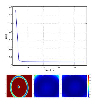
Figure 4. Root mean squared error between expected and observed codes as a function of the number of iterations of the calibration algorithm. The top plot shows the error averaged over all the pixels and poses, while the bottom pictures show for each pixel the error averaged over all the poses at iteration 0 (pinhole model), 2, and 21.
