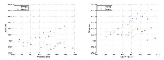
Figure 6. Scatter plot of the measured distances between pairs of points taken in the top part (left) and bottom part (right) of the target. The points where 620 target pixels apart.
